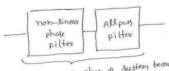
overall phase of system tecomes linear in pass band
